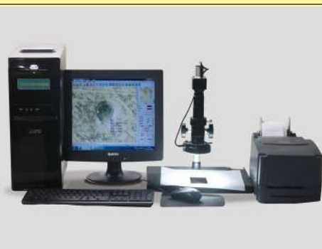
Electronic microscope measurement of the indent diameter (Ultimheat Laboratory)
